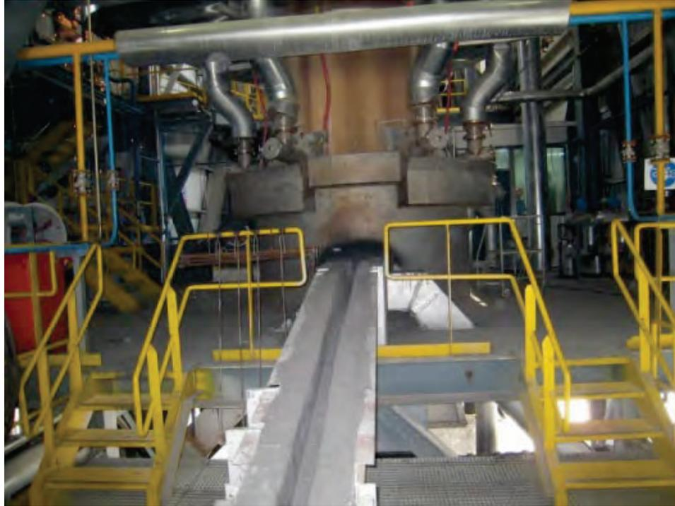
**Figure 3. Photograph of a turn-key cupola furnace (EC&S, 2019). The large cylindrical structure above the base is the cupola with tuyeres on its sides. Refined metal flows from the archway at the base down the ramp.**
